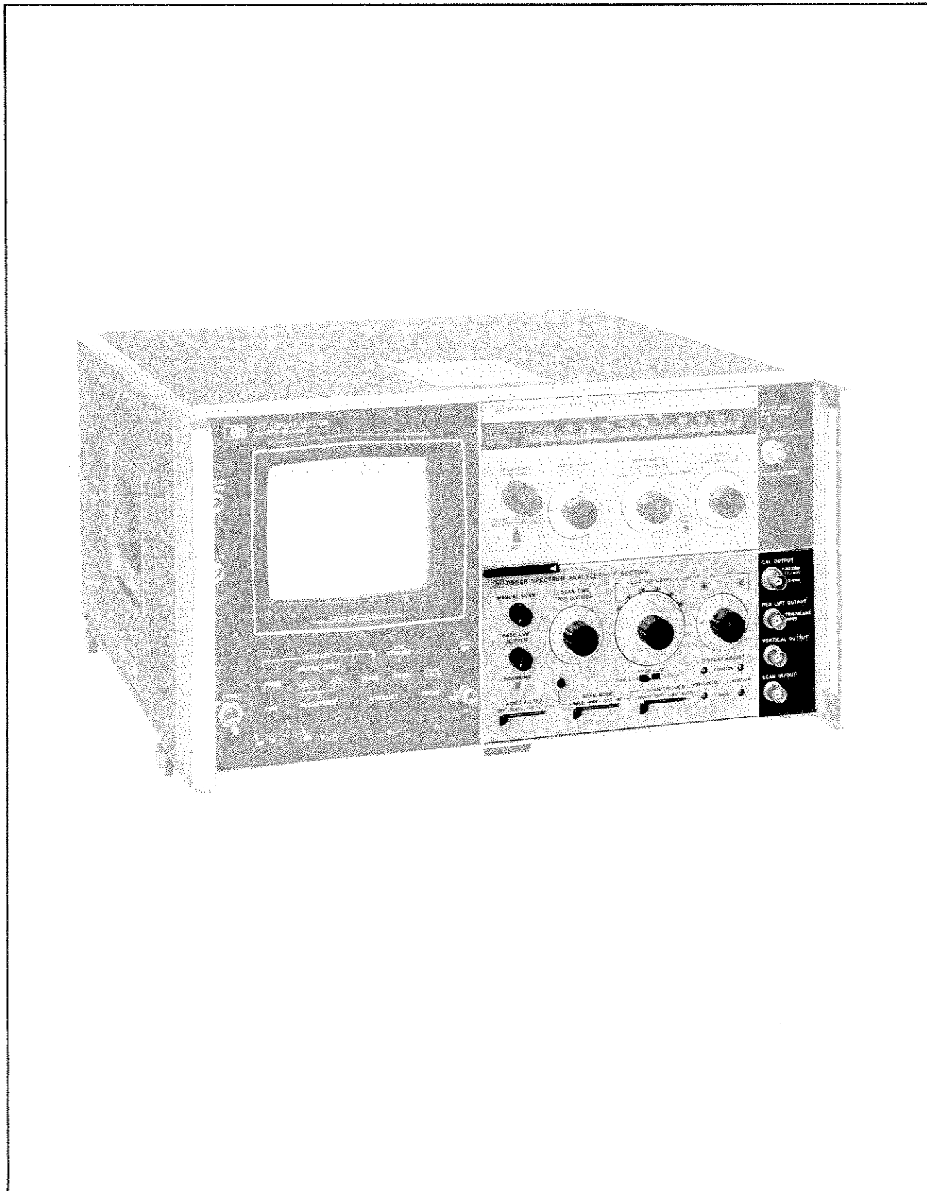
Figure 2-1. Model 8552B Spectrum Analyzer IF Section with 8553B RF Section and 141T Display Section
